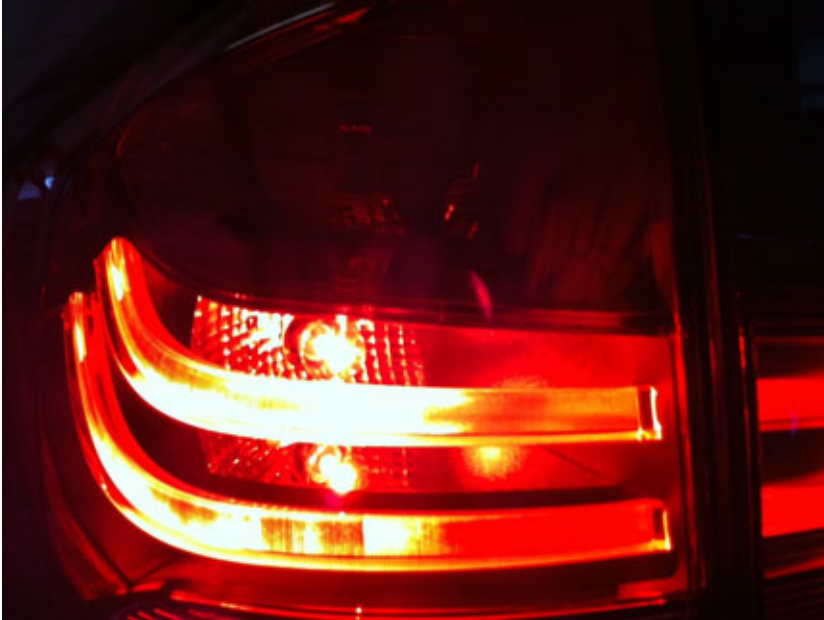
Two brake light bulbs located just behind the tail light LED tubes.
